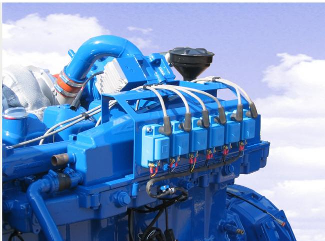
There are a number of ways to control engine ignition on large gas engines. This factsheet introduces inductive ignition systems, with a brief history and analysis of the major advantages of this type of system over other types of ignition system.
